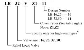
\* Use high-vent pressure types if the shifting time from unloading to on-loading is reduced.
