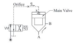
2) If logic valves are used at pressure above 200 Kgf/cm<sup>2</sup> maximum orifice diameters are limited.
